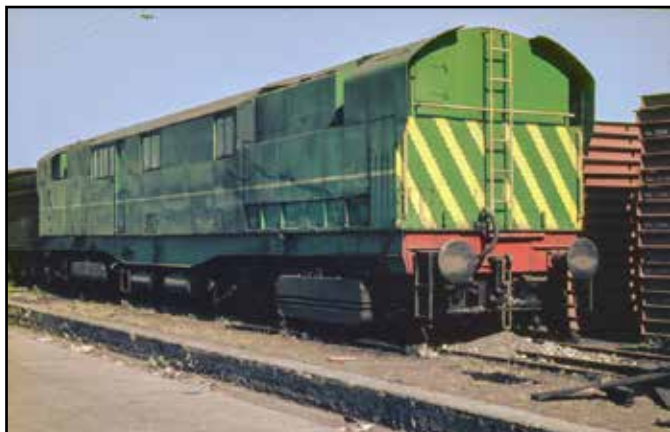
CIÉ turf burning locomotive CC1, Inchicore Works, 20 September 1959. (Photo © Tom Davitt - IRRS Archive)
