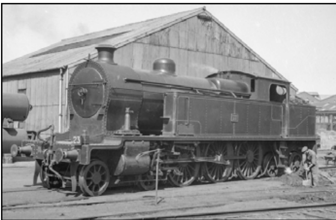
B&CDR 'Baltic' tank locomotive No. 23 at Queen's Quay, Belfast, circa 1953. (Photo © John Macartney Robbins - IRRS Archive)
